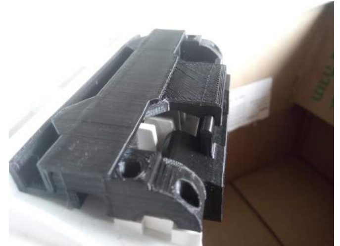
Photo 3: tab located in bracket groove
