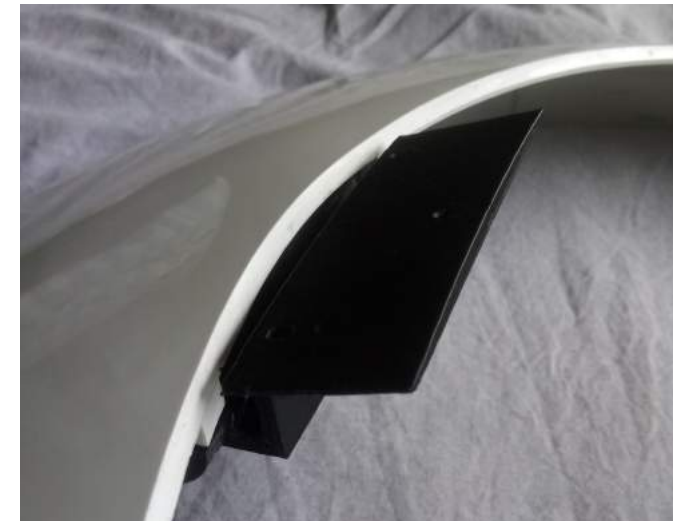
Photo 6: hinge installed and folded flat
